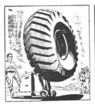
A tire that stands 10 feet high and 4 feet wide is described as the biggest in the world. It contains enough rubber to produce 3,200 passenger car tires and enough nylon cord for 7,000 pairs of ladies' stockings. Built by the Good-year Tire & Rubber Co., the tire is a research model of special-purpose tires for huge construction machines.
